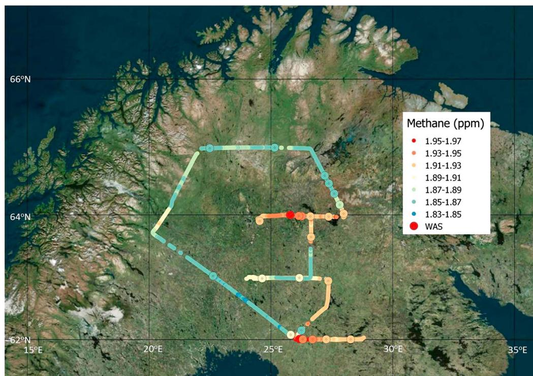
**Figure 7.** Map of methane mole fraction measured on the FGGA and in WAS bottles collected on flight B797 on 17 August 2013. Mean difference (WAS mole fraction – FGGA mole fraction) was  $-1.2$  ppb, within the FGGA measurement uncertainty. Mapped using QGIS 2.2.0 with basemap layer from Bing maps.
